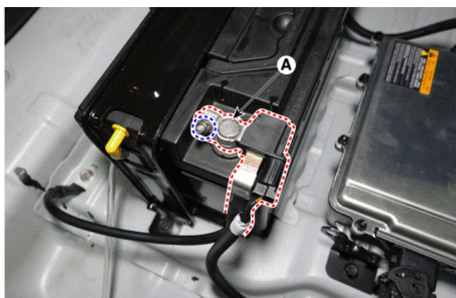
4-3. Turn the ignition switch OFF and disconnect the auxiliary 12 Volt battery negative (-) terminal (A).
