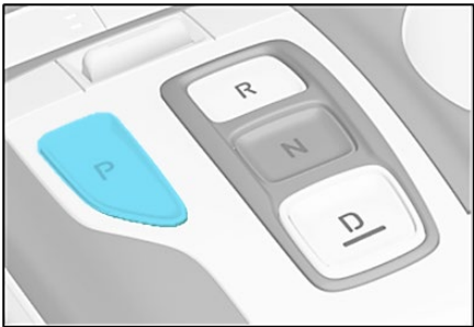
Step on brake pedal to park the vehicle, then select the shift button in park (P)
